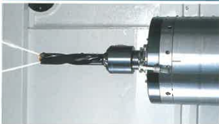
Through the Spindle (std.)
