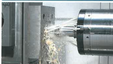
Flood coolant (std.)
