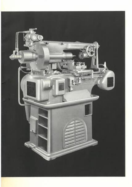
Blanks are automatically loaded through a hopper-feed system and are positively located and clamped on a solid arbor in cutting position. Cycle sequence includes rapid traverse to the cutting position, lowering the work slide to cutting depth, hobbing the gear, raising the work slide to clear the hob, rapid traverse away from the cut, and ejecting the gear. A new blank is loaded automatically, and the cycle is repeated continuously until the machine is shut off.
