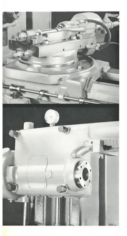
swivel. The hob drive pinion and drive shaft have tapered roller bearings. Spiral bevel gears reduce the noise and allow the hob drive to be reversed by changing the leads to the motor. All running surfaces are automatically lubricated by the Bijur system. Wear strips on the end support can be replaced rather than replacing the complete support. The standard swivel is adjustable from 60° right to 90° left. The vernier indicating dial is graduated to 10' for accurate setting.
