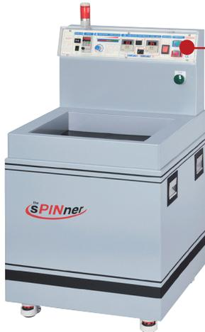
Each sPINner includes adjustable speed & intensity controls with programmable timers for each direction.
