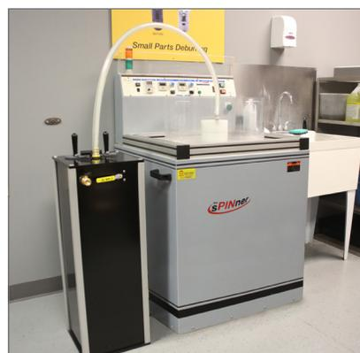
Filtration unit continuously cleans deburring fluid, minimizing machine downtime for water changes.
