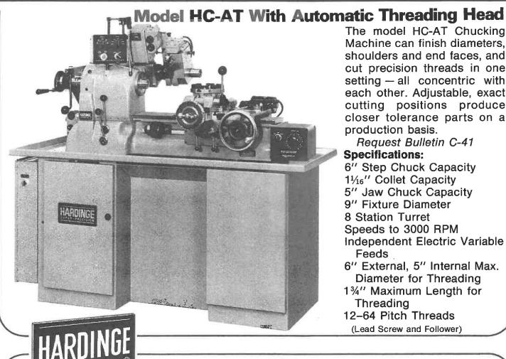
The model HC-AT Chucking Machine can finish diameters. shoulders and end faces, and cut precision threads in one setting - all concentric with each other. Adjustable, exact cutting positions produce closer tolerance parts on a production basis.
