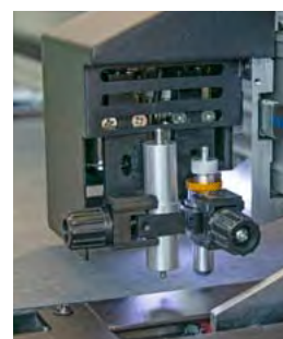
Dual tools head delivers 1kg of force per tool
