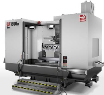
The **EC-1600ZT-5AX** includes the integrated 4th-axis platter, and adds a 5th-axis rotary and A-frame support for full 5-axis machining of large parts.
